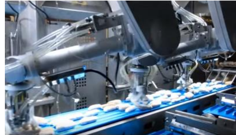
Robots pick and place ice cream bars for subsequent packaging. (Courtesy of JMP Automation, Inc.)
